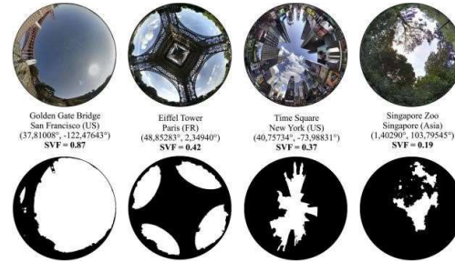
Figure 10 Skyview Factor derived from Fish eye camera
