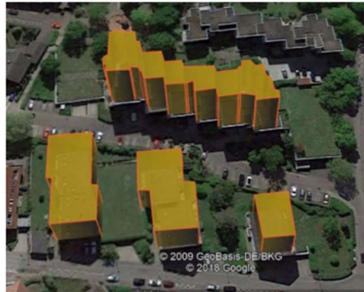
Figure 25 LOD2 3D Buildings generated from Open Source Software (Jayaraj and Ramiya, 2018)
