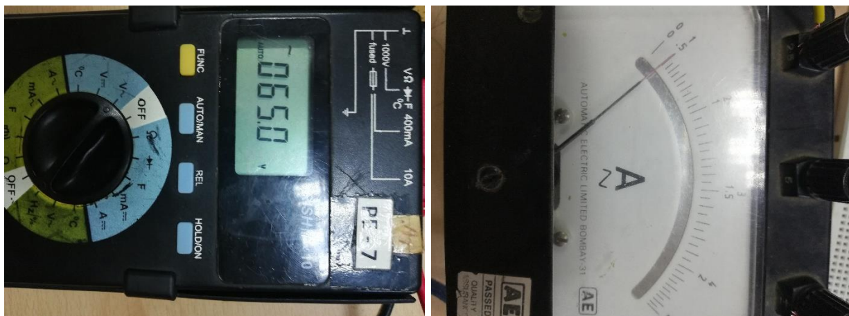
Fig 3: Voltage and current measurement readings from meters for V=65V and I=0.5A
